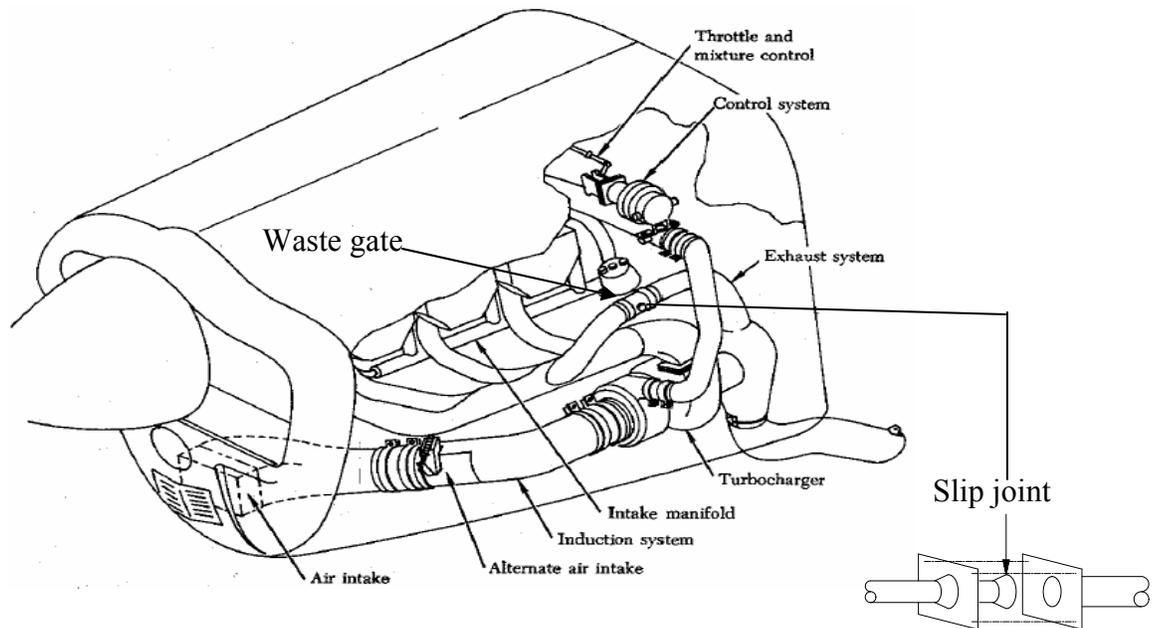
Figure C-5. Six-Cylinder, Horizontally Opposed Turbocharged Engine [C-1]
