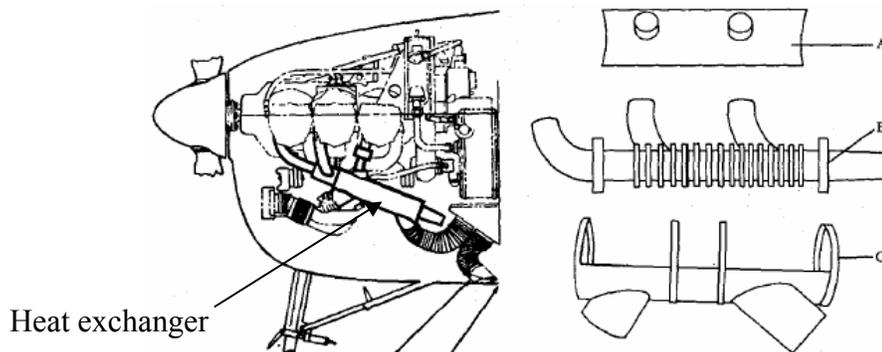
Figure 1. Six-Cylinder, Horizontally Opposed Reciprocating Engine [5]
