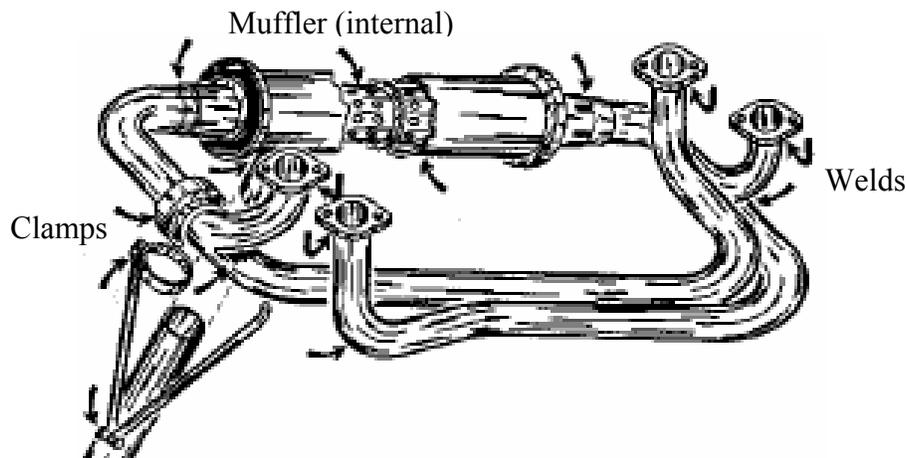
Figure 2. Typical Exhaust System Inspection Areas [5]
