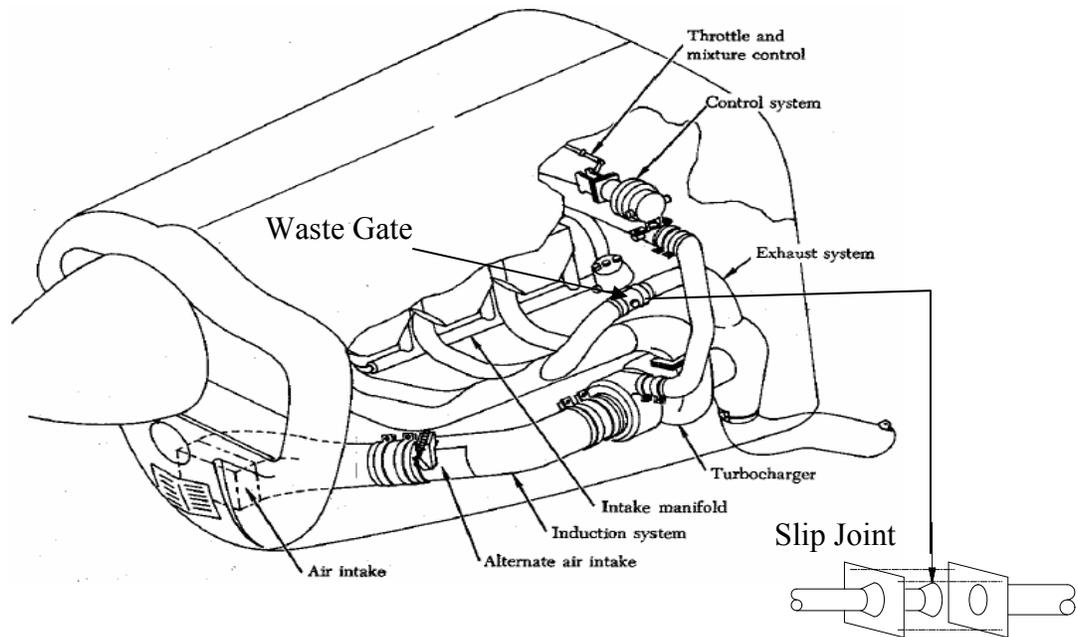
Figure 5. Six-Cylinder, Horizontally Opposed Turbocharged Engine [5]
